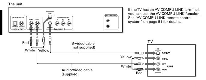
Connect the unit to a TV equipped with stereo audio input and video input jacks using the supplied audio/video cables.
